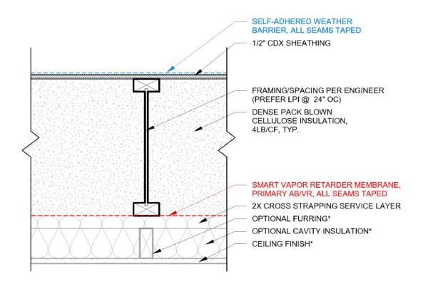
**1X4 STRAPPING** WEATHER BARRIER, **ALL SEAMS TAPED** FRAMING/SPACING PER ENGINEER (PREFER LPI @ 24" OC) DENSE PACK BLOWN CELLULOSE INSULATION, 4 LB/CF, TYP. 1/2" CDX PRIMARY AB/VR, ALL JOINTS TAPED 2X CROSS STRAPPING SERVICE LAYER OPTIONAL FURRING\* OPTIONAL CAVITY INSULATION\* **CEILING FINISH\***
